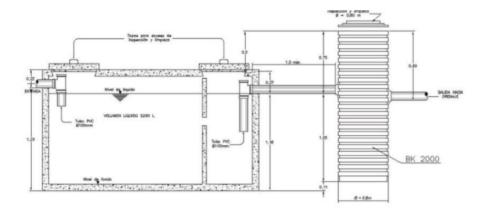
4) The FAFA upflow filter that is currently required for an efficient system, called the Enhanced Septic System.
