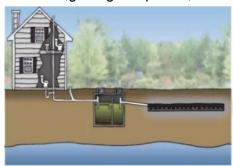
Septic tanks can be built of cement, plastic or fiberglass. These septic systems are always buried, with a location spacing of at least 1.5 meters from the foundation of the building.
