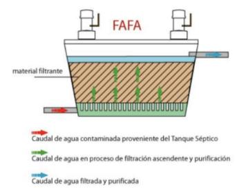
The basic operation consists of the entry of wastewater into the septic system, where the first stage is responsible for retaining fats, then light solids.
